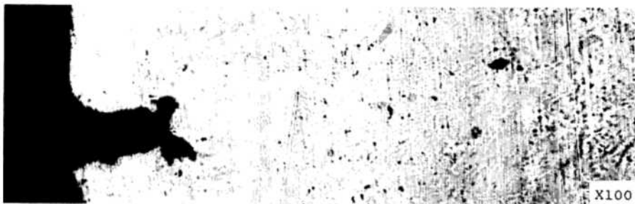
Fig. 12 Optical micrograph of the shape of the apparent plastic zone near the end of the notch
